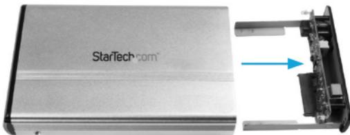
2. Align the SATA connector on the hard drive with the connectors on the rear panel and connect them together. Ensure the SATA drive is sitting squarely between the rails:
