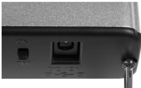
7. Once the drive has been secured within the Enclosure, connect the DC power adapter to the DC power port. Connect the remaining end of the power adapter to an available electrical outlet.
