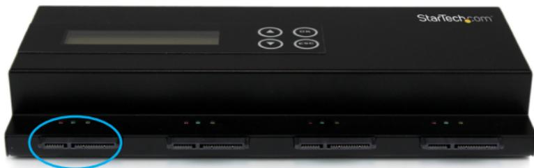
3. Using an included SATA Cable, connect up to 3 HDDs you would like to have overwritten, or erased to the destination ports. (3 ports from right to left, see below)
