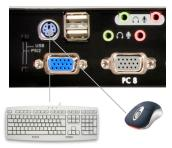
PS/2 Keyboard and USB Mouse: The mouse slide switch must be switched to the right, while the keyboard slide switch must be switched to the left.
