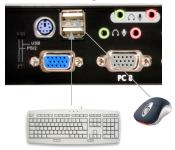
Please note: When configuring the switch as a slave in a cascaded configuration, PS/2 Keyboard and Mouse is the only mode that can be used. As such, SV431DUSB cannot be configured as a slave in a cascaded setup, as it does not provide a slide switch selector.
