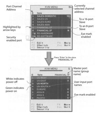
By hitting the left <CTRL> key twice within two seconds, you may see the 'Hotkey Menu' if it is enabled (an OSD option). Or, by hitting the left <CTRL> key three times within two seconds, you will see a 'KVM MENU' screen displaying a list of the computers with corresponding channel addresses, names and status.
