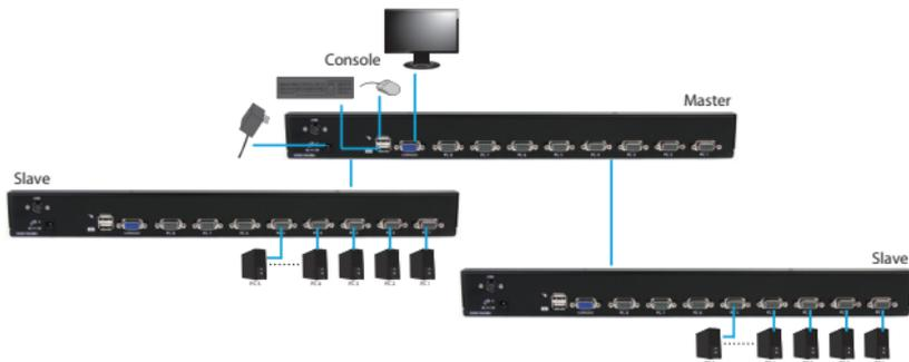
**NOTE!** A device (computer or KVM switch) at any 'PC x' port can be changed at any time after initial power-up. If you change any one of the PC 1 to PC 8 port connections from a computer to a Slave KVM switch or vice versa, or replace the devices of a port, the OSD will update this change the next time it is activated.
