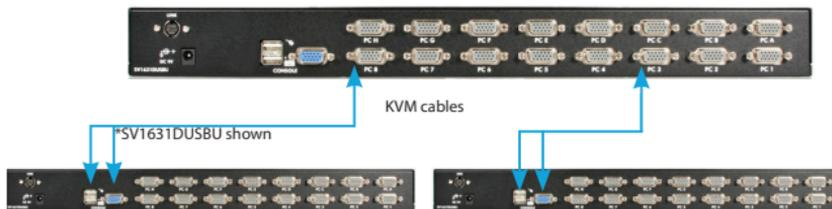
The maximum number of computers controlled by a Master/Slave configuration with all 8-port KVM switches used is 64, with 8 Slaves and each Slave connecting to 8 computers:
