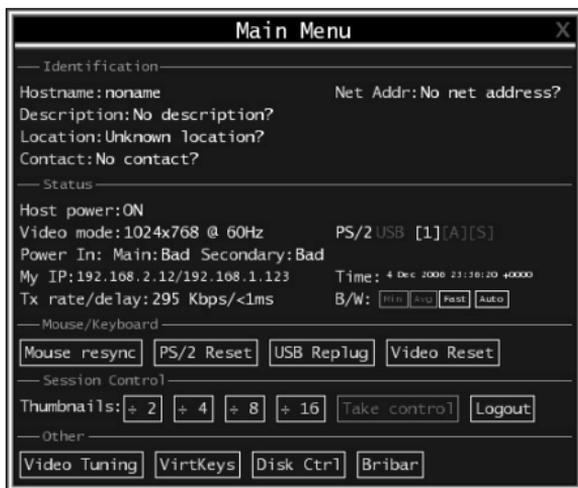
The main menu window may be moved by clicking and dragging on the title bar. It can be closed by pressing Escape, or by clicking on the red X in the top right corner. Here is a guide outlining various fields from the Main Menu. Most of the functions operate immediately. Other functions require a response to a confirmation prompt first before performing the requested function.
