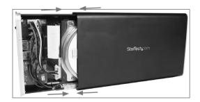
5. Re-fasten the Base Stand to the base of the Enclosure and replace the screw removed in Step #1. Drive installation is now complete.
