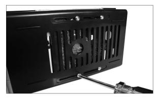
4. Slide the Disk Mounting Tray (with drive attached) back into the Enclosure, so that the Enclosure is sealed.
