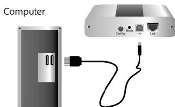
3. Position the Remote unit where you want it. Connect the Cat5e, Cat6, or Cat7 patch cable to the Link port (RJ45) on the Remote unit and to a network switch or wall network port connected to a switch. Connect the Remote unit to a power source.
